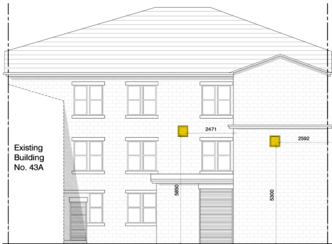
Figure 2 Extraction Syetm on West Elevation
