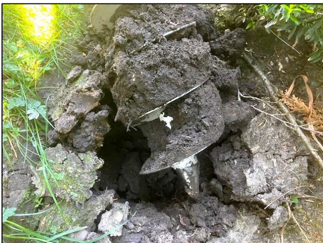
Plate 3. A borehole indicating that the soil is dark and loamy, well-draining and has very low clay content.
