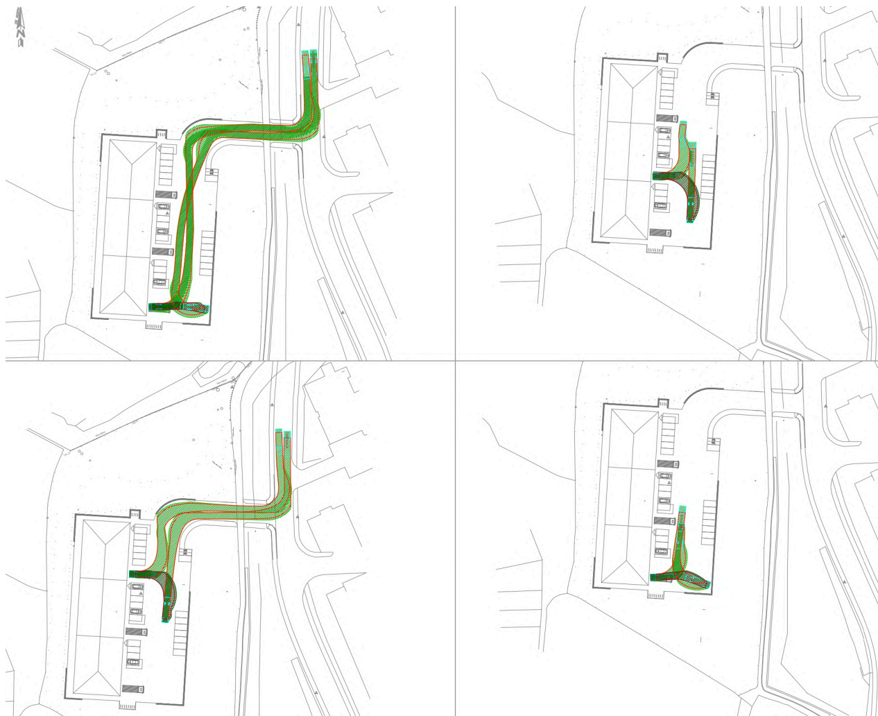
Figure 3.2 : Swept Path Analysis – 10m Rigid HGV & 11.2m Refuse Collection Vehicle
