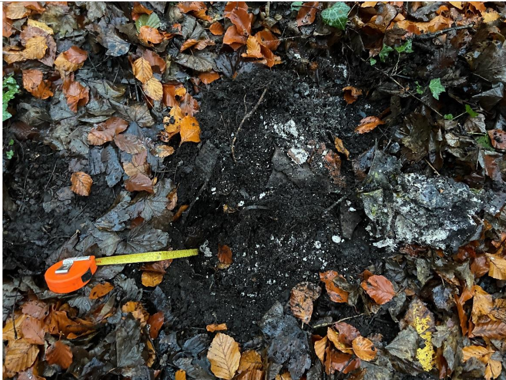
PLATE 6 HP105 EXCAVATION WITH VISIBLE ASBESTOS FRAGMENTS
