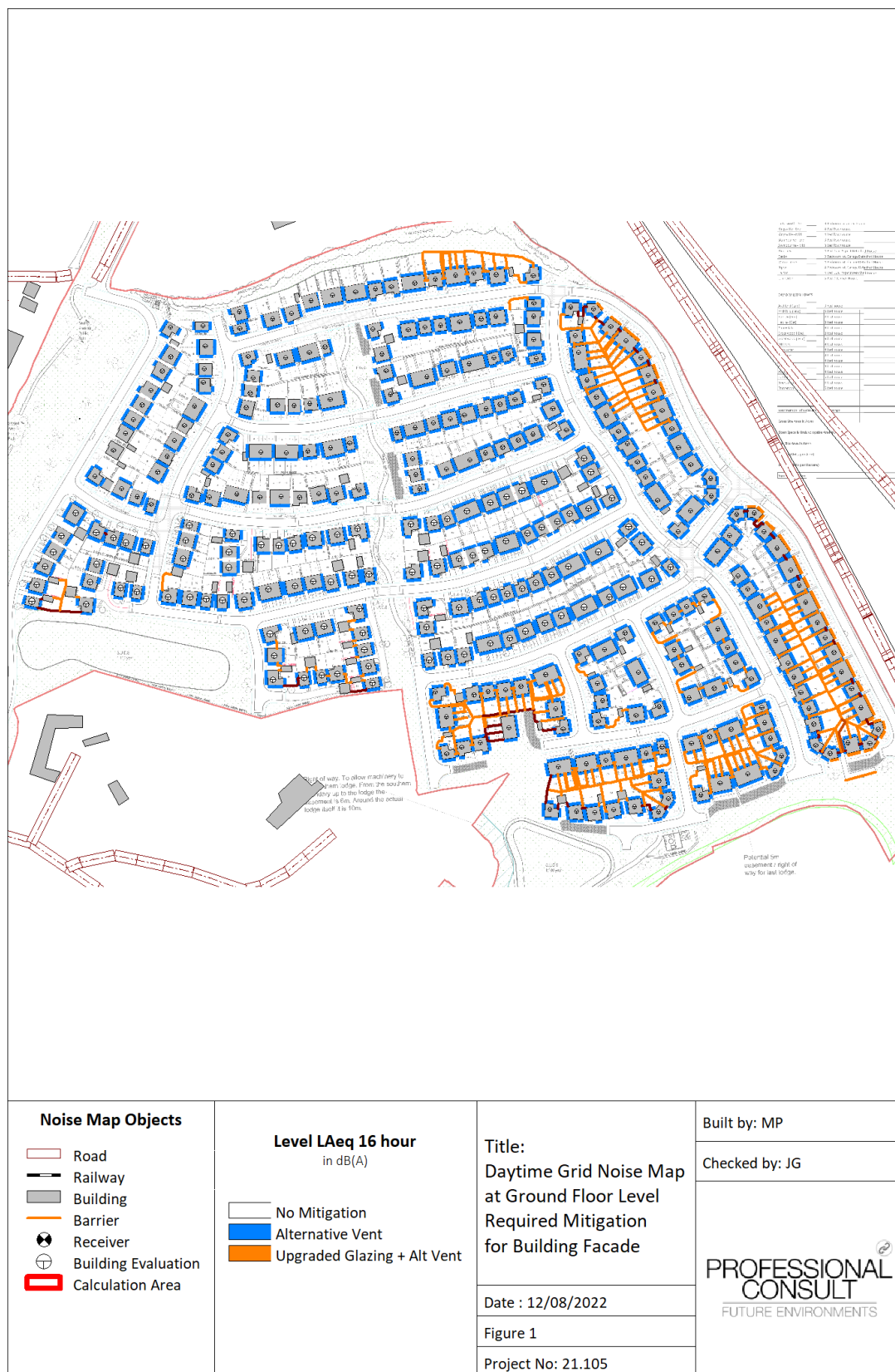
Figure 1 Daytime Grid Noise Map – Require Mitigation for Building Façade – Ground Floor
