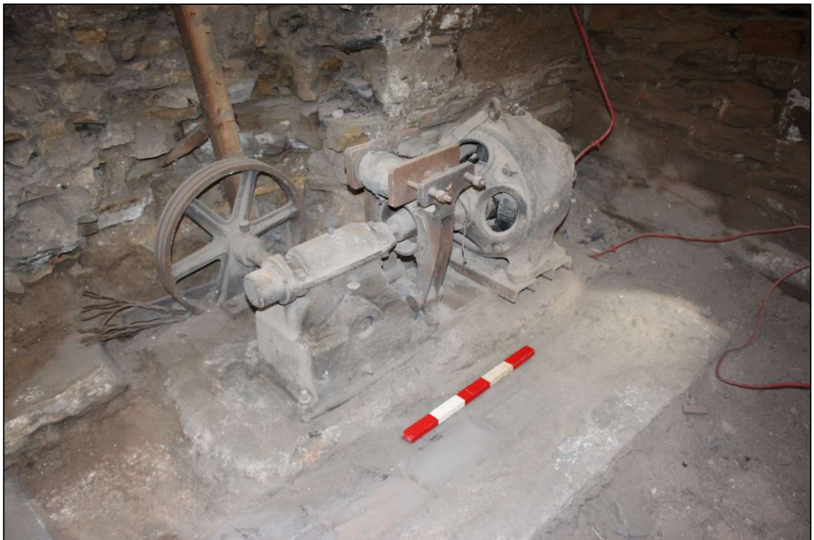
Plate 10: The electric motor that powered the dumb-waiter
