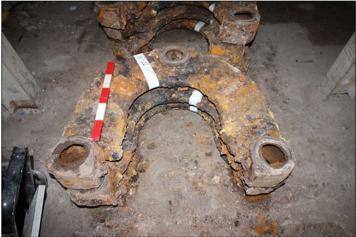
Plate 12: Detail of the cast-iron sections of the saddle boiler
