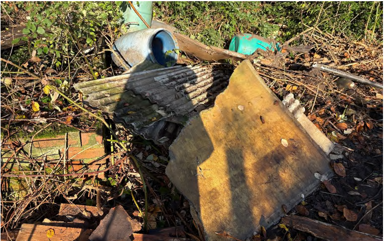
Figure 2 – Asbestos Cement Panels
