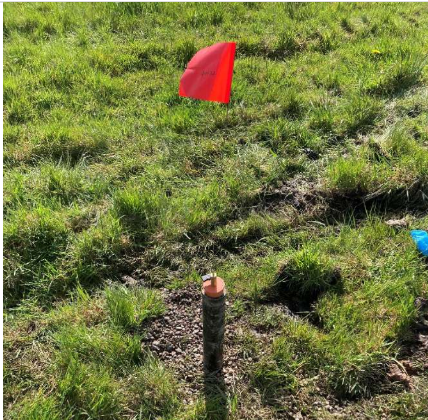
PLATE 4 WINDOW SAMPLE MONITORING WELL
