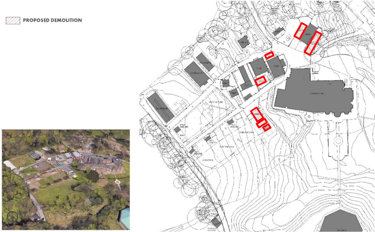
Figure 6.2 Proposed Demolition Plan (Seven Architecture, 2024)
