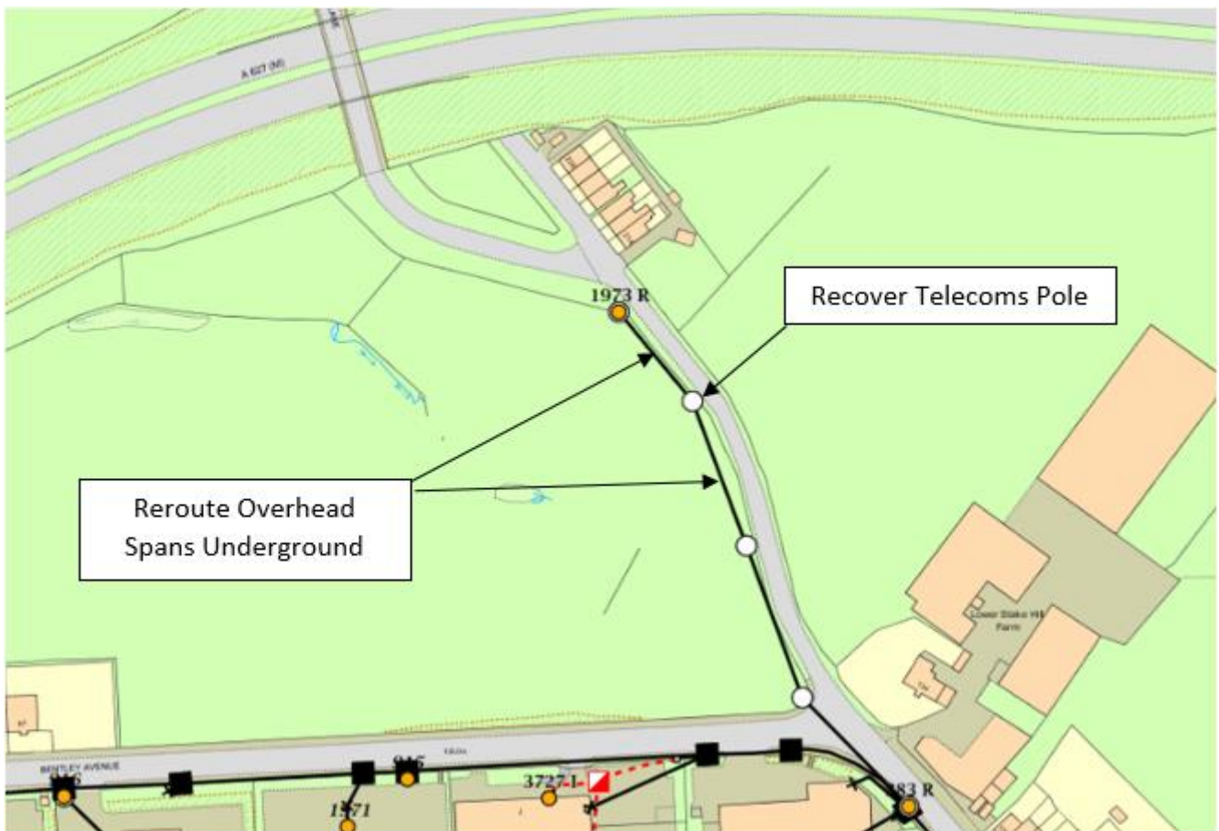
Figure 5.2 – Existing Openreach Apparatus to be diverted
