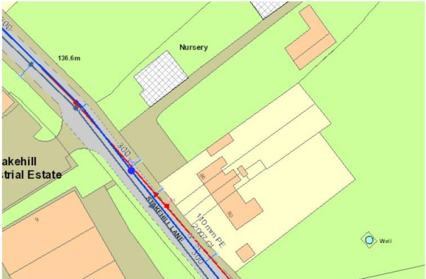
Figure 4.2 – Water Service Disconnection
