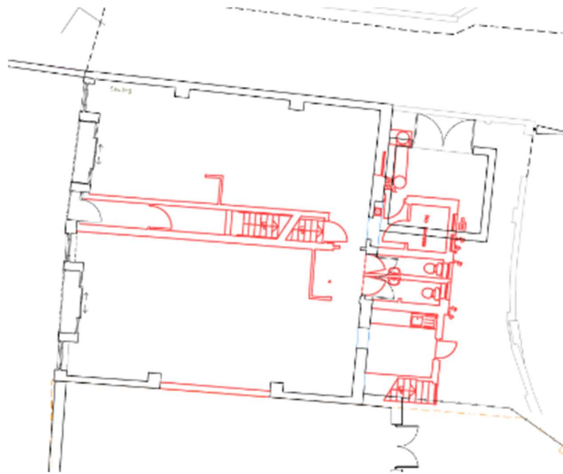
Figure 30 – Architect's GF Demolitions Plan
