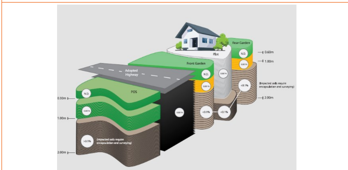
FIGURE 9.1 ASBESTOS RISK MITIGATION CONCEPTUAL SITE MODEL
