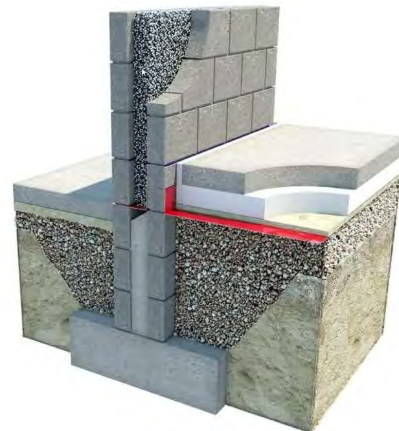
Figure 5 - Typical foundation make up with split level
