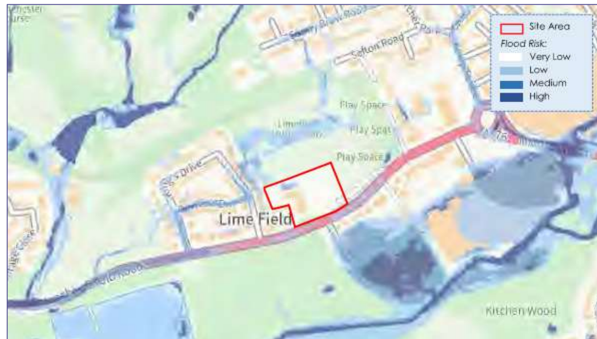
Figure 8 - Surface Water Flooding to Site (FRA)
