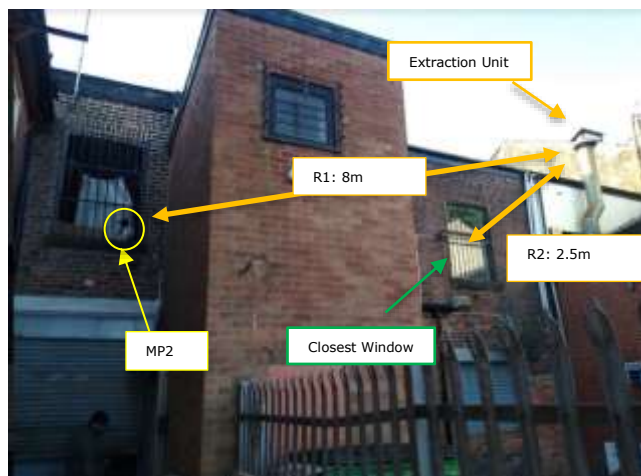
Figure 4.0 – Rear Façade and distance correction
