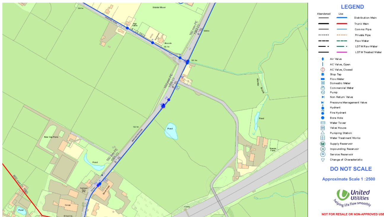
Figure 2: Existing Fire Hydrant Locations
