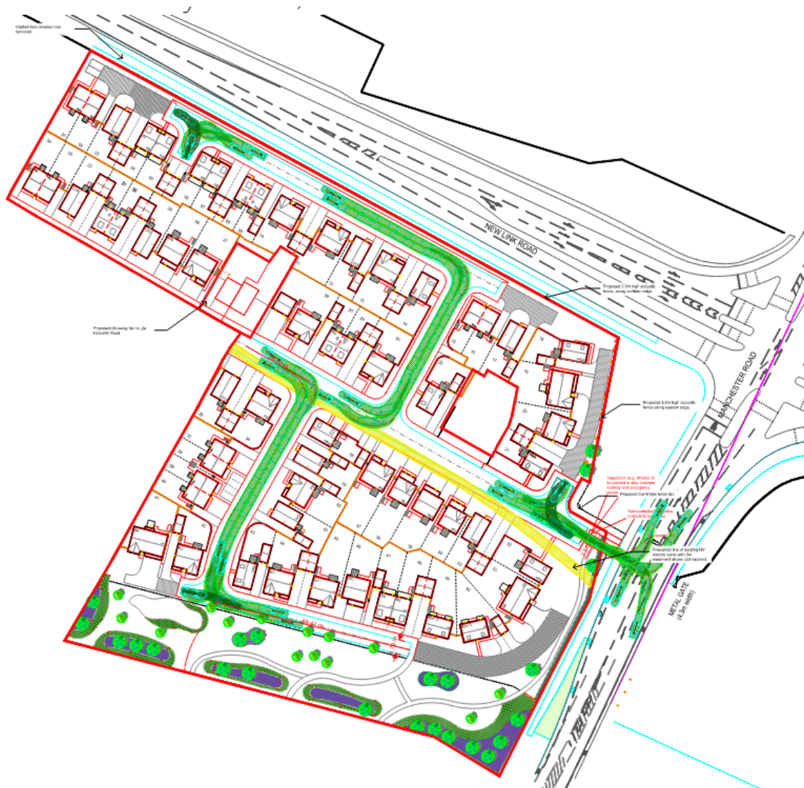
Figure 4: Fire Service Access – Track Layout
