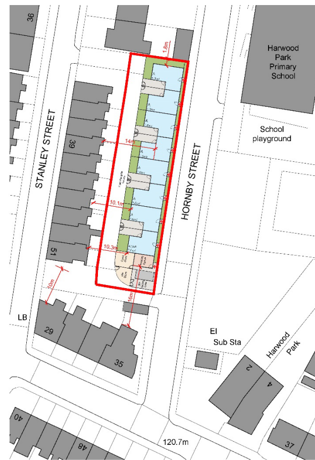
Figure 12: RIBA Stage 2 Design Option 2 (one-storey)
