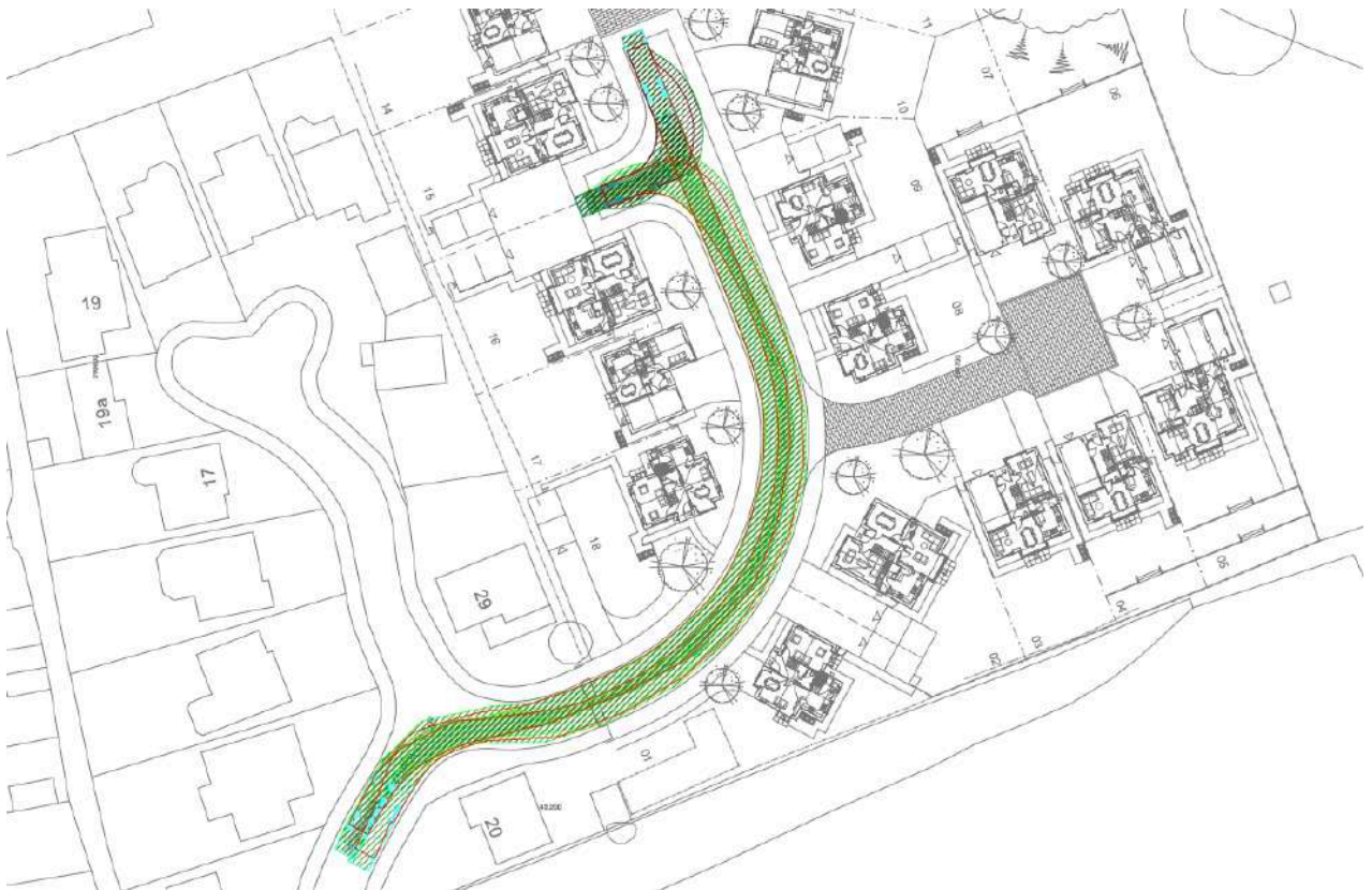
Figure 3.2 : Swept Path Analysis – 11.2m Refuse Vehicle
