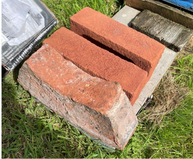
Figure.2 Brick sample next to example of existing brickwork.
