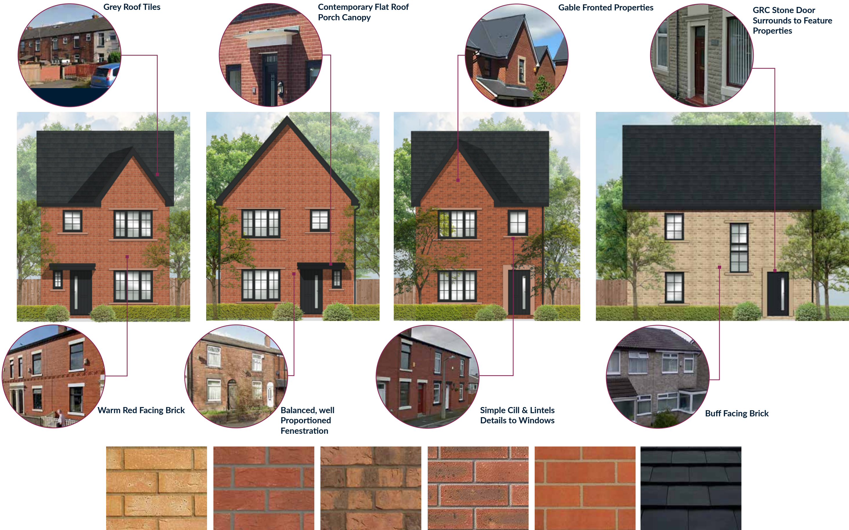
Fig 4.1 | Building Materials & Detailing
