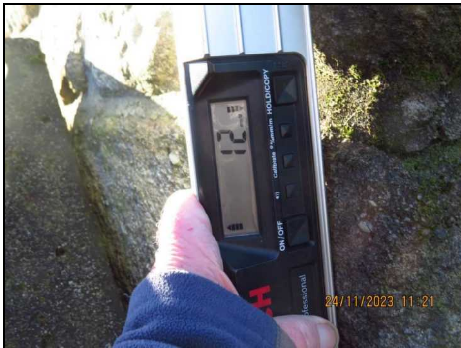
009 Vertical alignment \pm 6mm per metre
