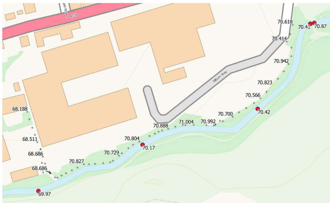
Figure 4 – Comparison of bank levels and flood levels for the 1 in 100 (1%) flood event. Contains Ordnance Survey data © Crown copyright and database right 2020
