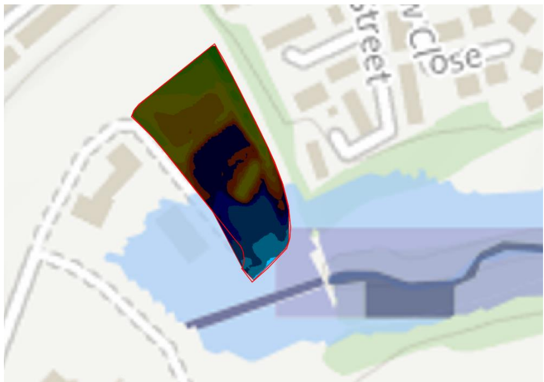
Figure 8: Flood Level Analysis using LiDAR – 133.500m AOD
