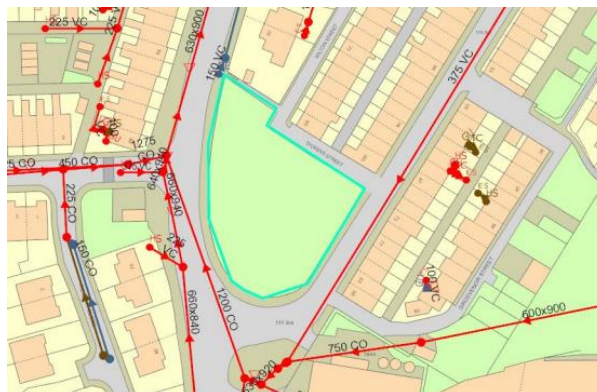
Figure 3: UU Sewer record extract
