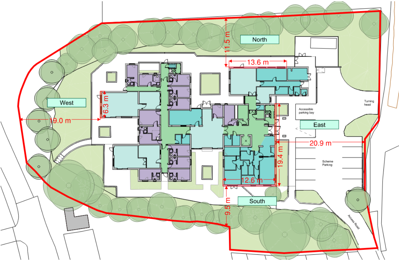
Figure 17: Elevation references to site boundary.
