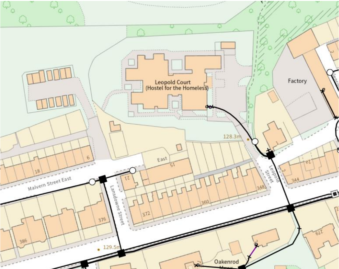
Figure 8.1 – Existing Openreach infrastructure
