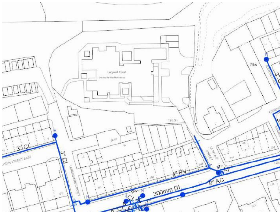
Figure 7.1 – Existing water infrastructure plan
