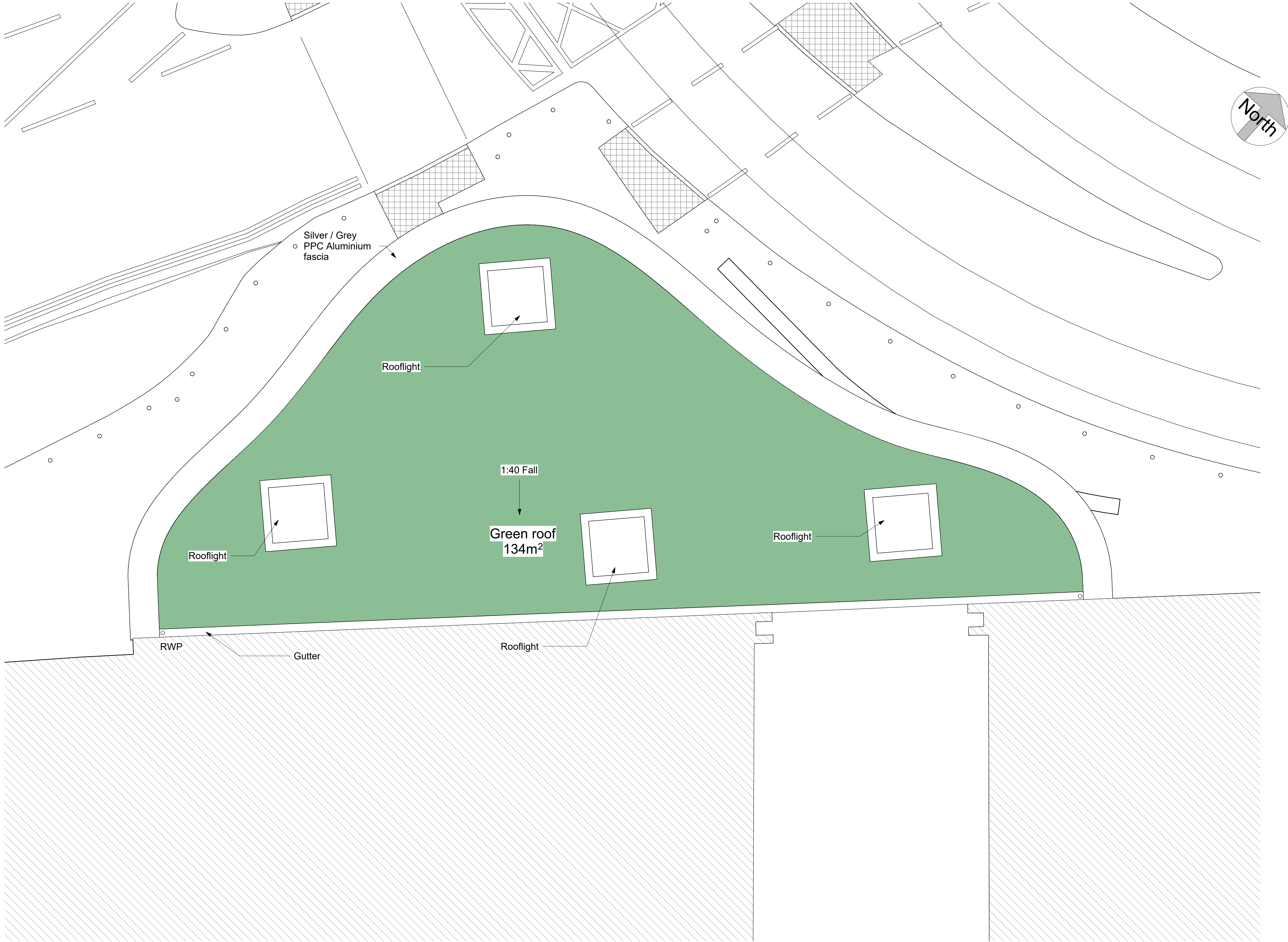
1 Forecourt Works - Roof Plan 1 : 50
