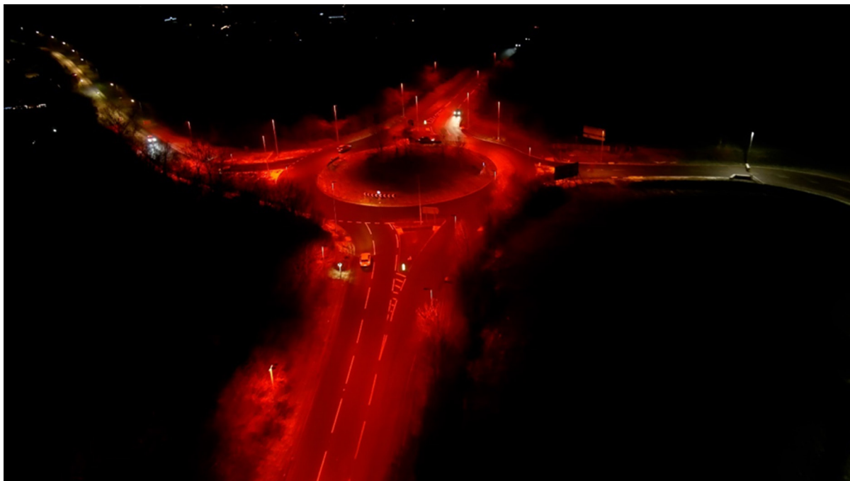
Photo 10: Red spectrum lighting install, A4440 Trotshill Way, Worcester.
