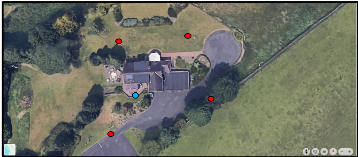
Figure 2: Location of surveyors (with IR Cameras ●) over the survey period and standalone IR camera position (●).
