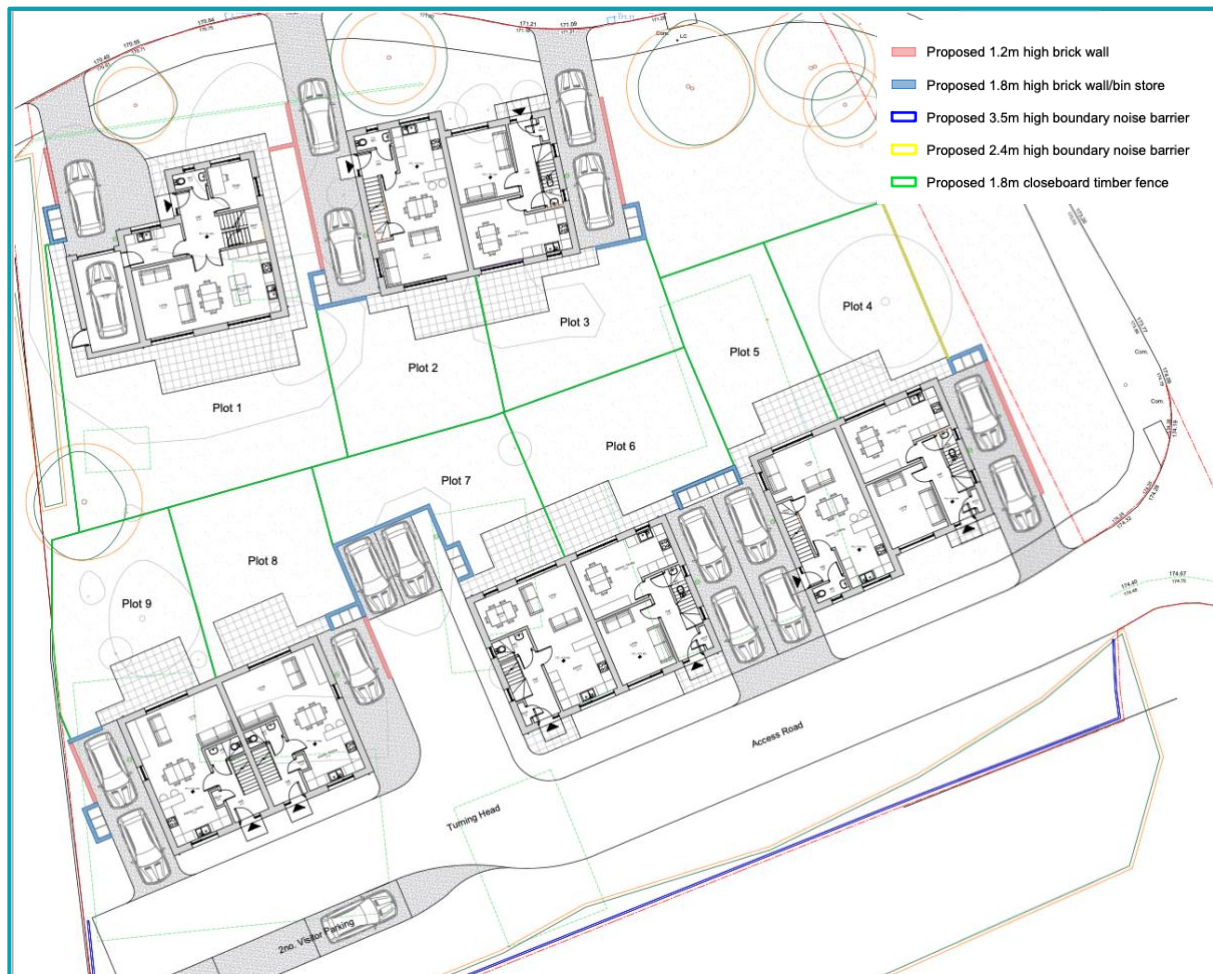
Figure 1.1 Site Plan & Boundary Treatments
