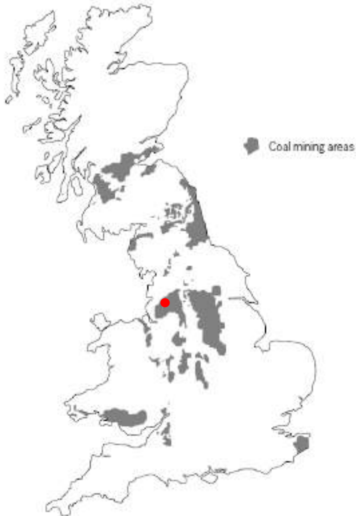
Figure C3 Coal mining areas of Great Britain where sulfate bearing, coal mining wastes and metal processing slags are most likely to be encountered
