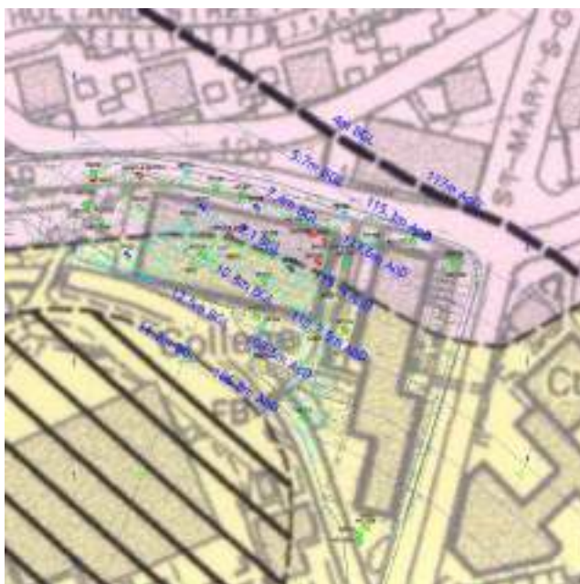
Figure 8-1 Depth of Arley Mine Throughout the Site
