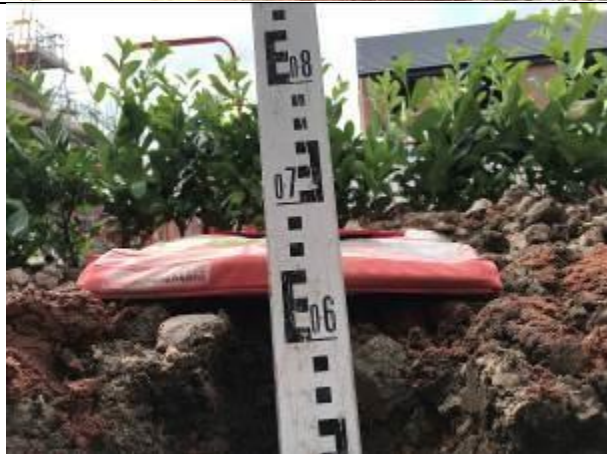
Depth measurement in garden area to the front of Plot 1 ( circa 640mm).
