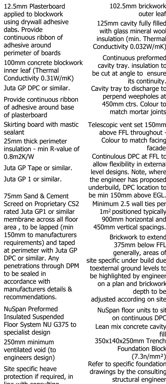
Brick External Wall / Ground Floor Junction Max External Ground Level
