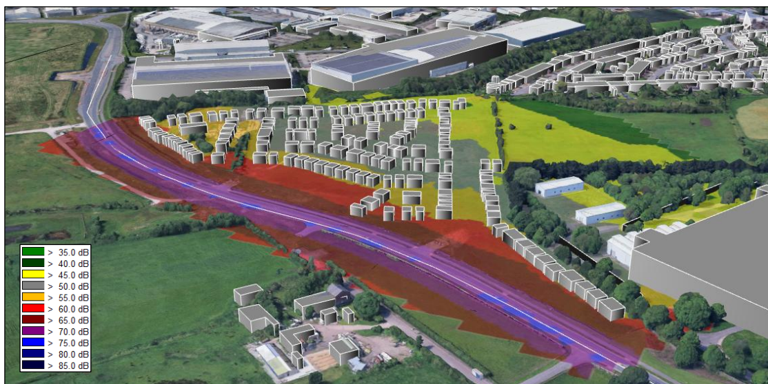
Screenshot of CadnaA model predicted road noise impact during the daytime (07:00-23:00)
