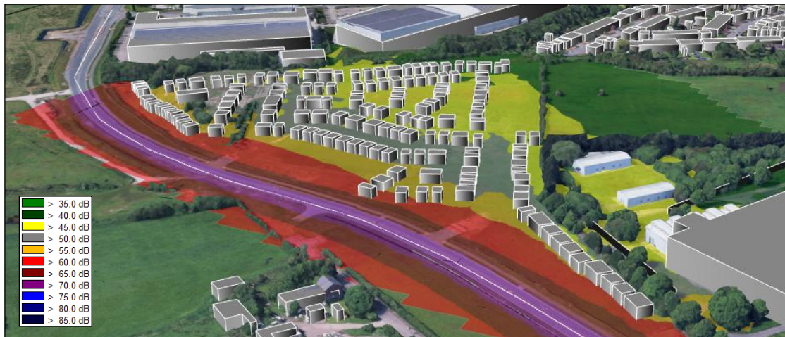
Screenshot of CadnaA model predicted road noise impact during the nighttime (23:00-07:00)
