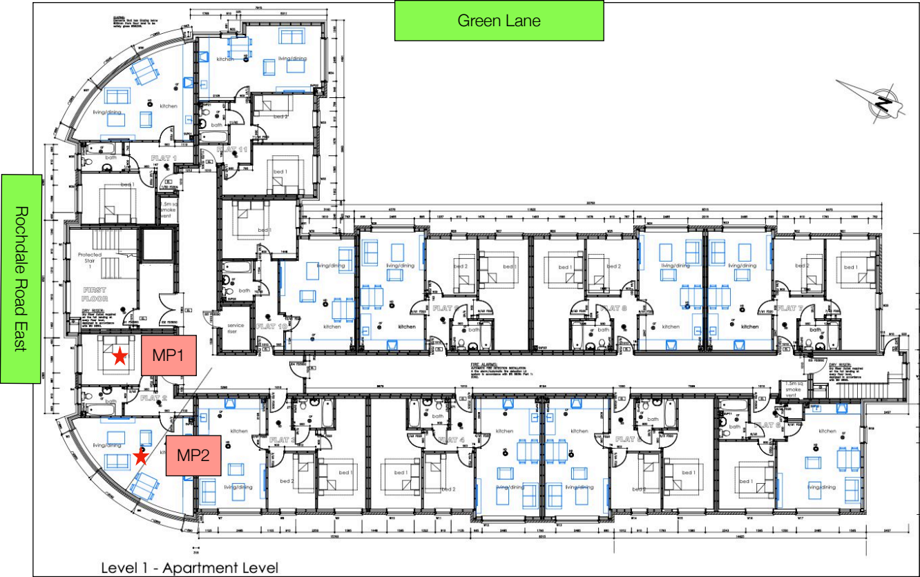
Figure 3.1: Internal Ambient Sound Measurement Positions - 1st Floor
