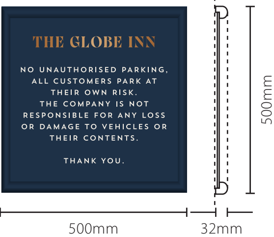
Scale : 1:10 @ A3 Item H. 1no. Powder coated aluminium car park disclaimer. G/CI - 1400mm D - 32mm
