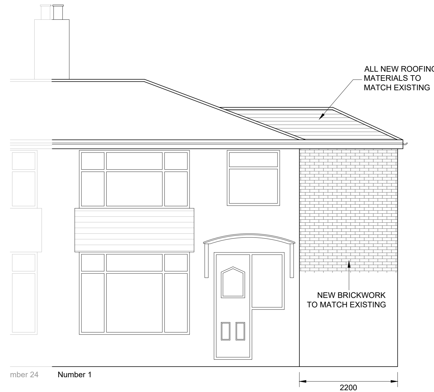
PROPOSED FRONT ELEVATION (SCALE: 1:50)
