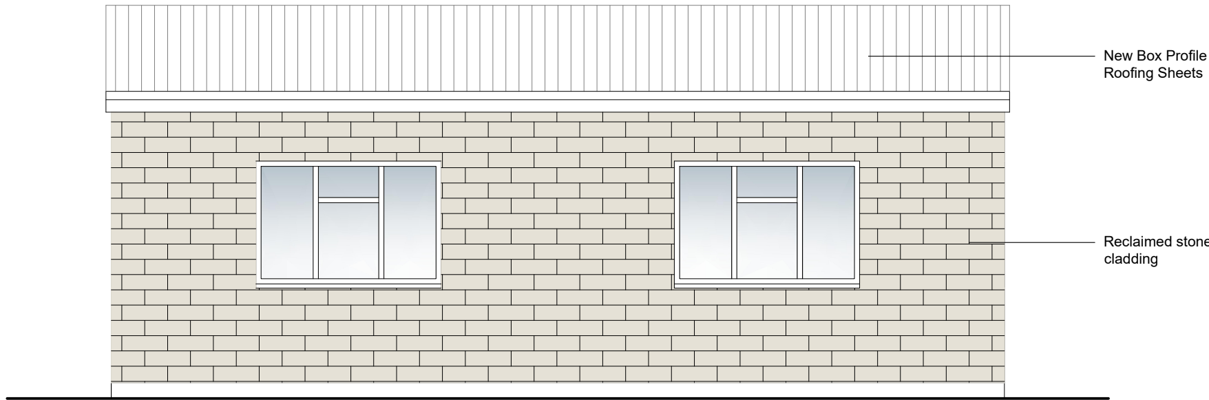
APPROVED SIDE ELEVATION 1
