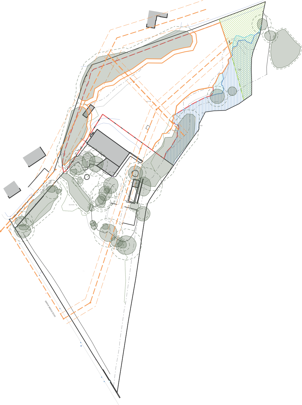
10m offset from the River Roch, root protection area of trees within developable area, and existing sewers with easement zones
