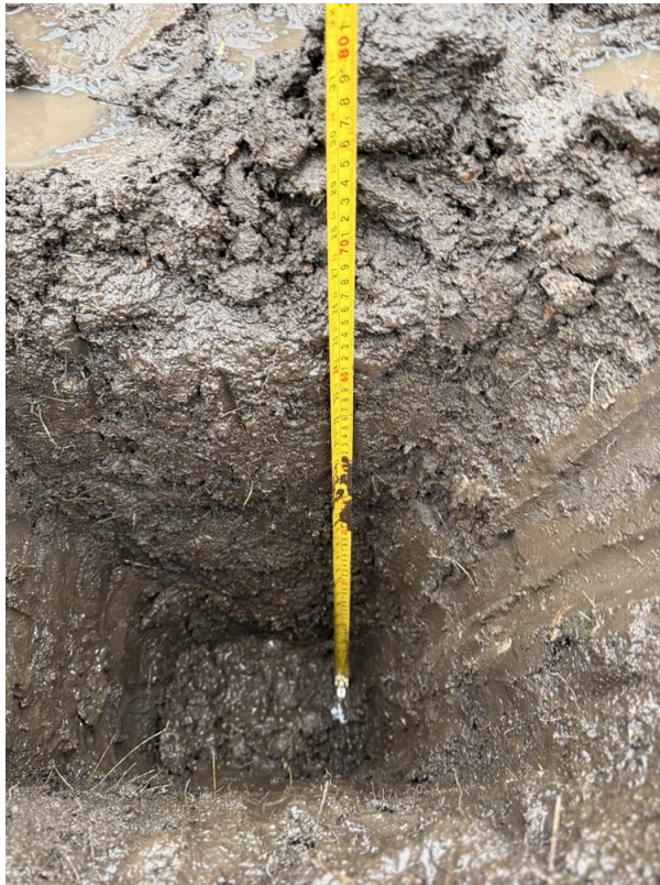
Photo 11 Plot 60 300mm capping layer
