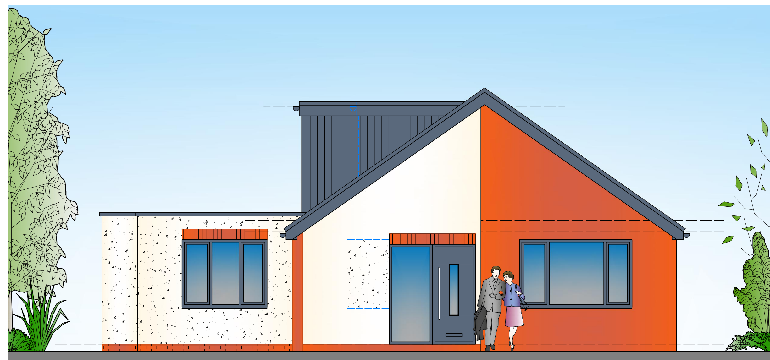
PROPOSED FRONT ELEVATION scale 1:50
