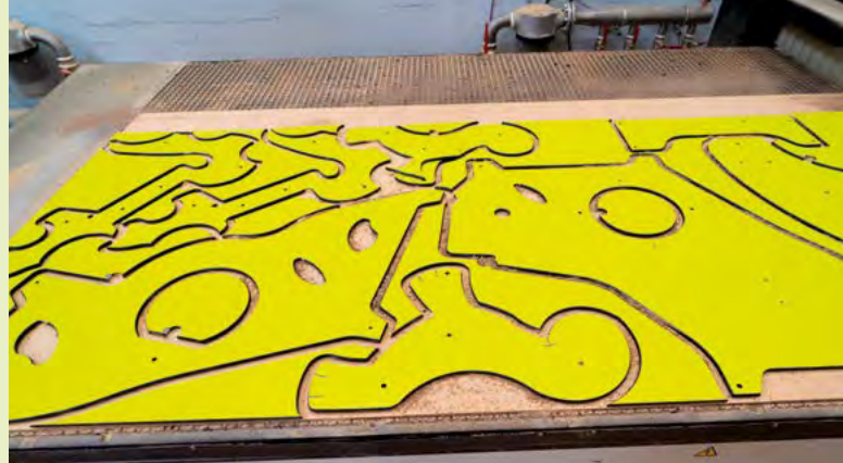
We optimise the cutting of panels to limit leftover scraps.
