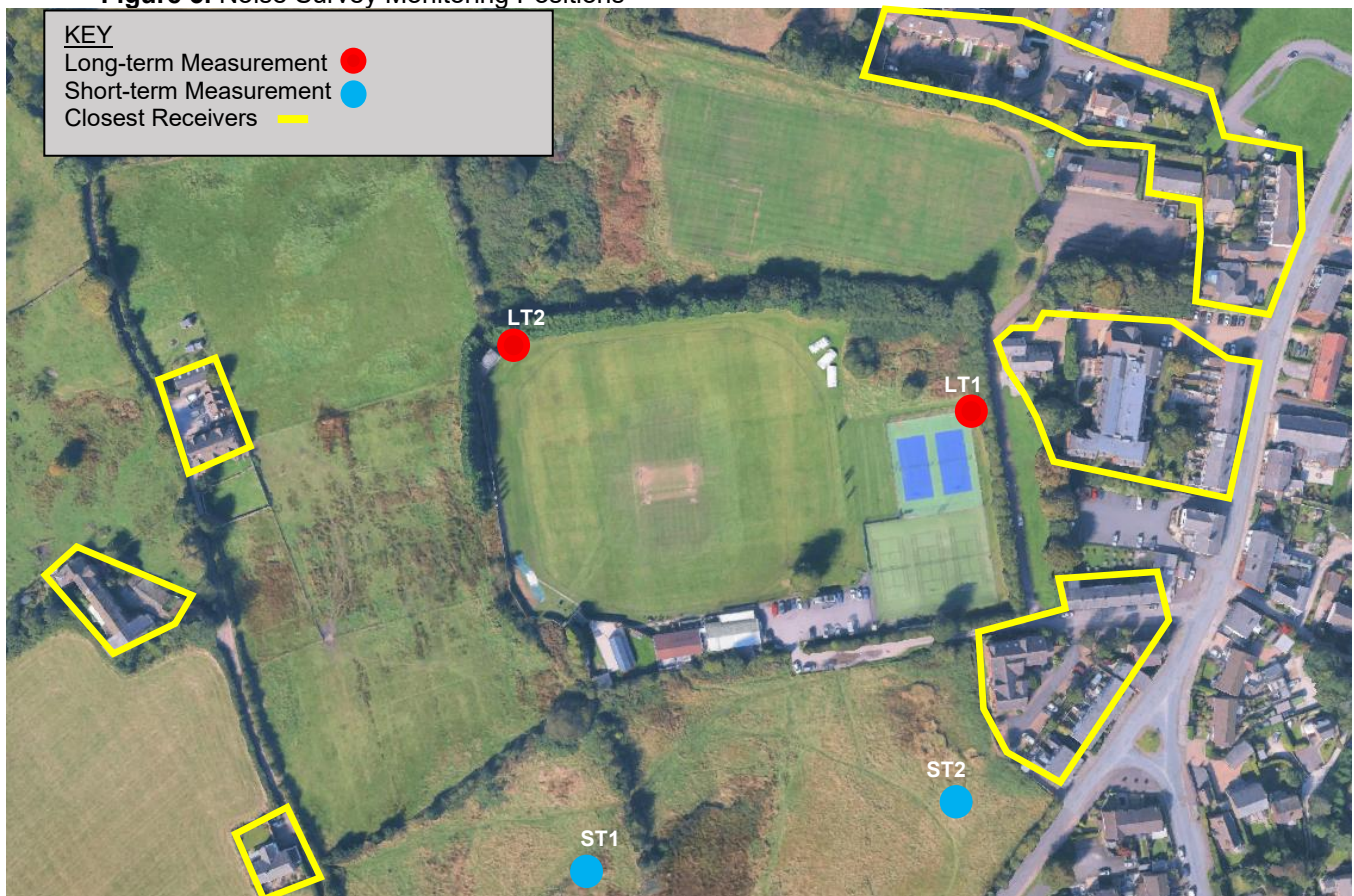
Figure 3. Noise Survey Monitoring Positions
