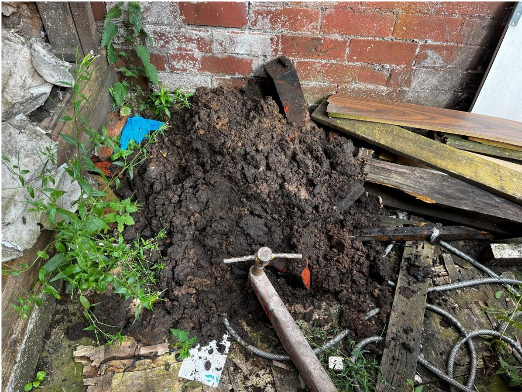
Plate 1 – Window Sampler Borehole 01 (WS01) ground level (gl) to 1.20m below ground level (bgl).
