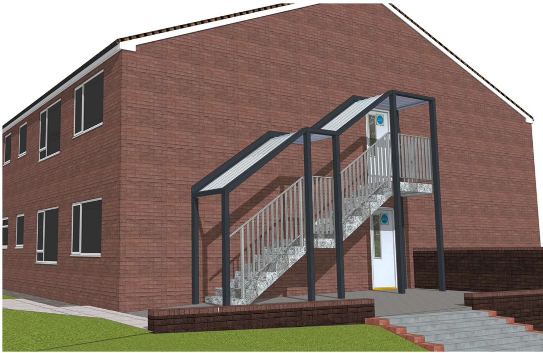
Above – typical view of canopy protection to staircase
