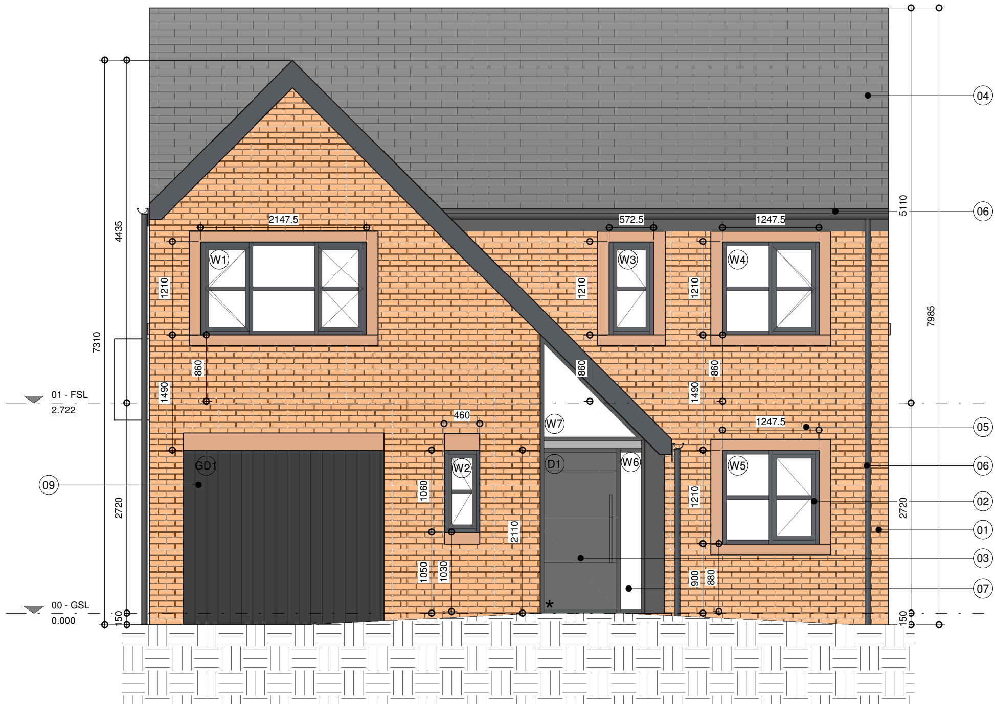
Front Elevation Plot 06 Scale: 1 : 50
