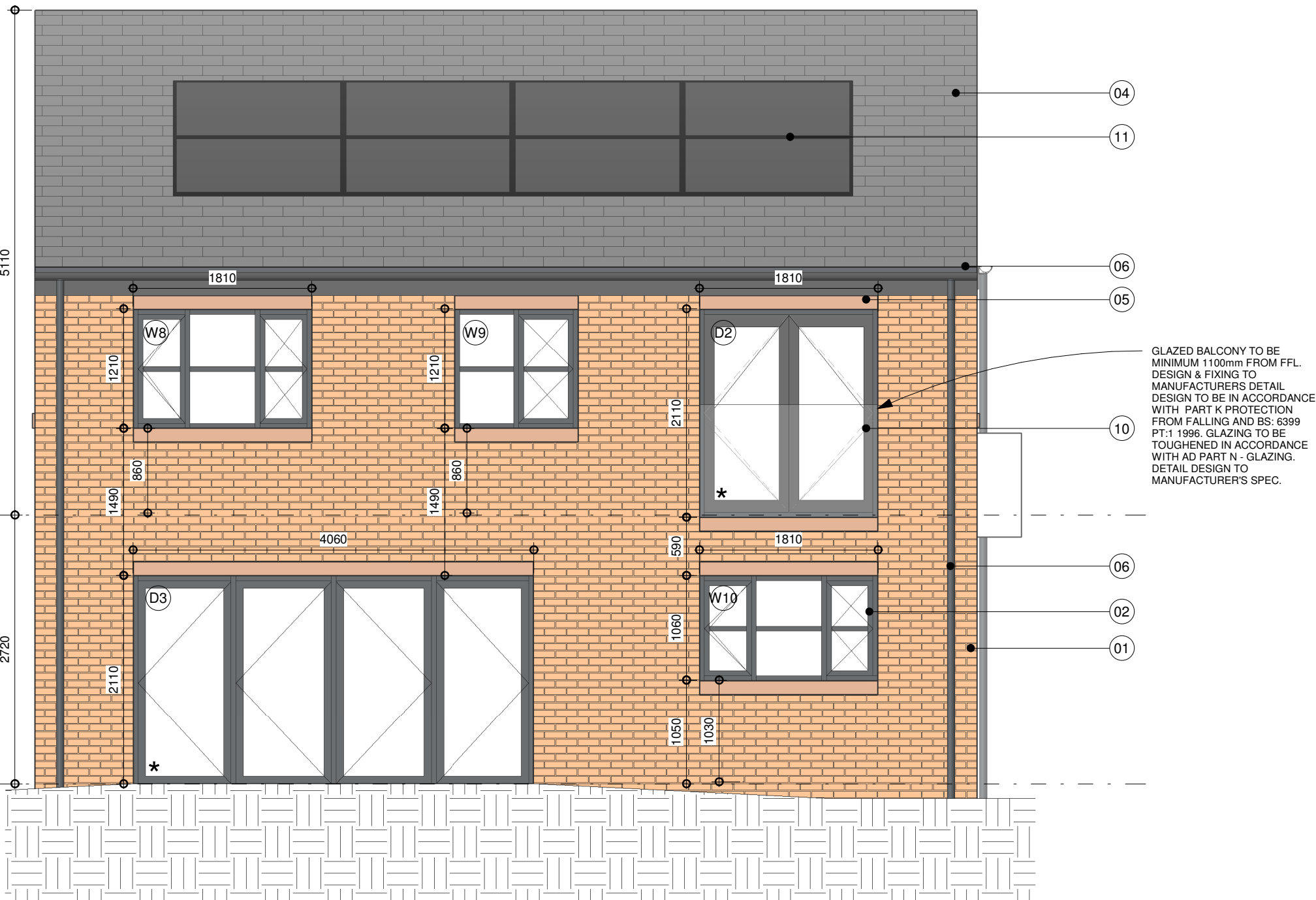
Rear Elevation Plot 06 Scale: 1 : 50
