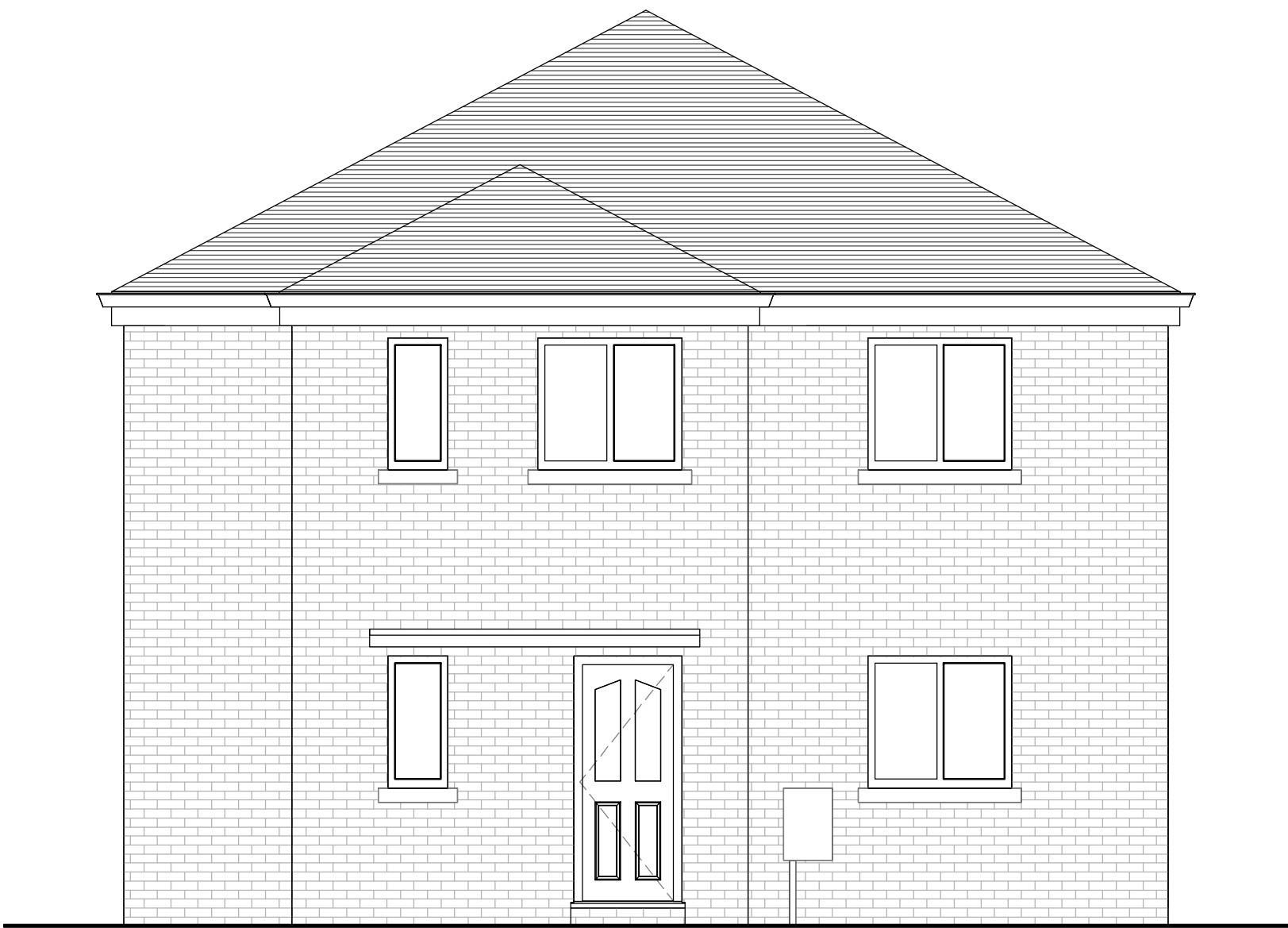
Existing Front Elevation 1 : 50
