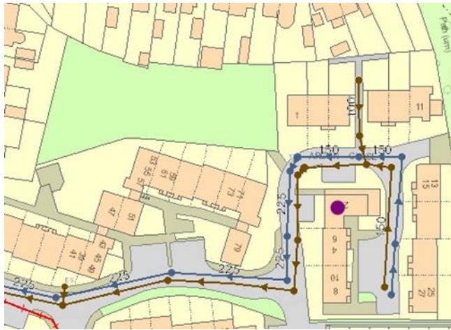
Fig 1. Screenshot of UU sewers. Blue = SW and Brown = Foul Sewer
