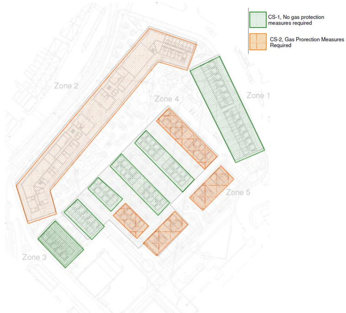
Figure 3.1 Extract From Curtins' Proposed Ground Gas Protection Measures Zoning Plan (Proposed Layout Has Been Superseded)
