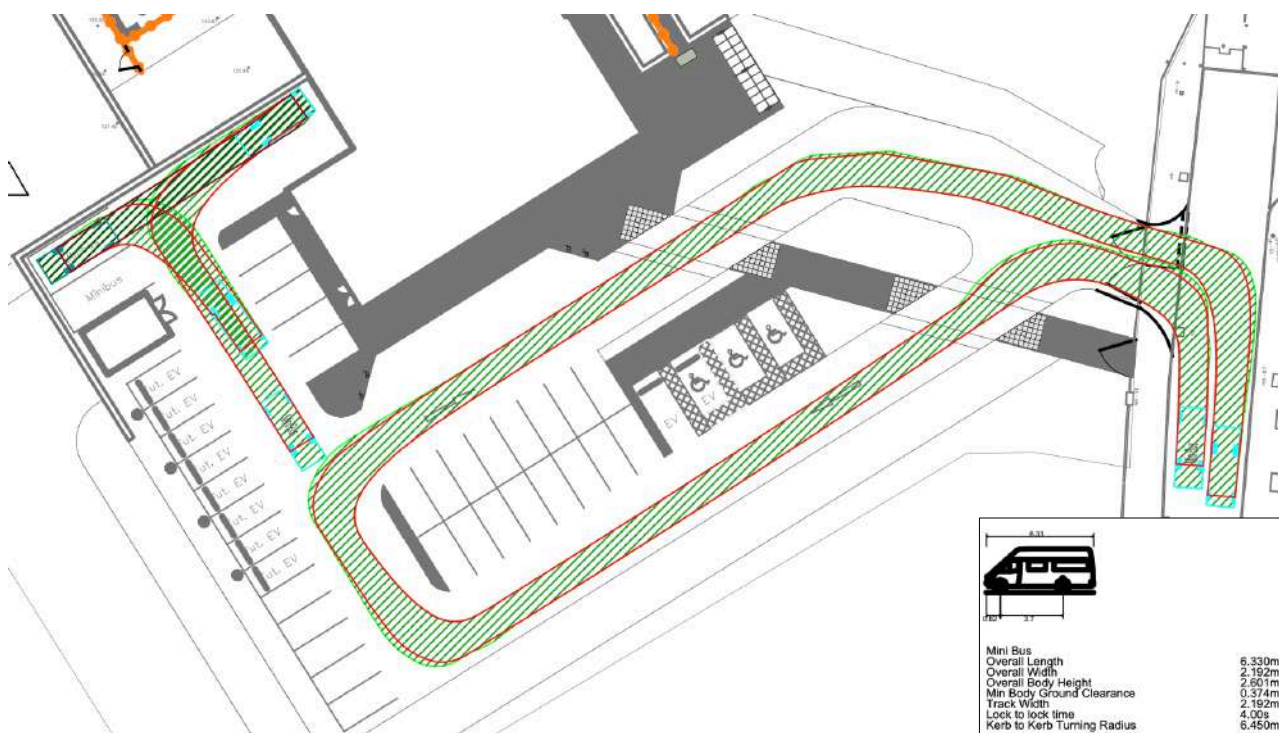
Figure 4.5 : Swept Path Analysis – Fire Appliance (8.6m)
